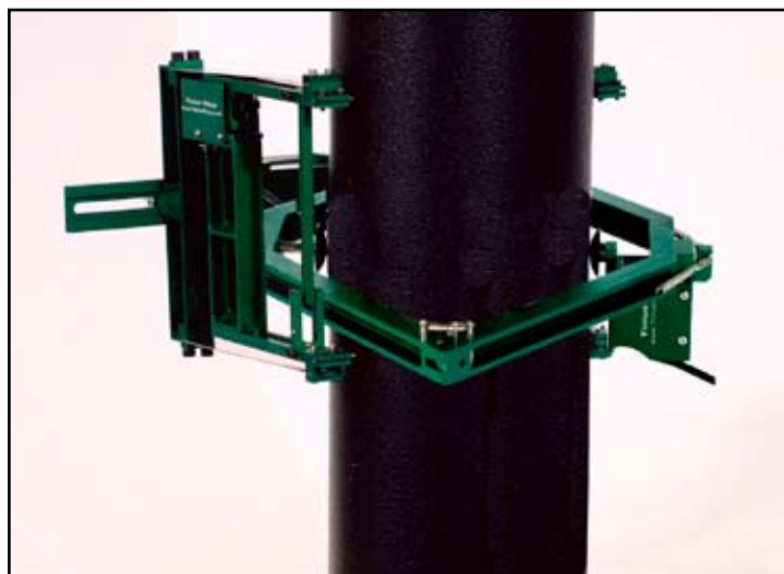
Figure 2. Model 3542RA extensometer may be used simultaneously with the model 3975 diametral extensometer (shown) or model 3544 circumferential extensometers.
