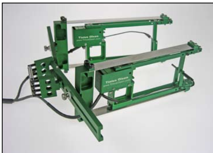
Figure 1. Model 3542RA2 averaging axial extensometer.
