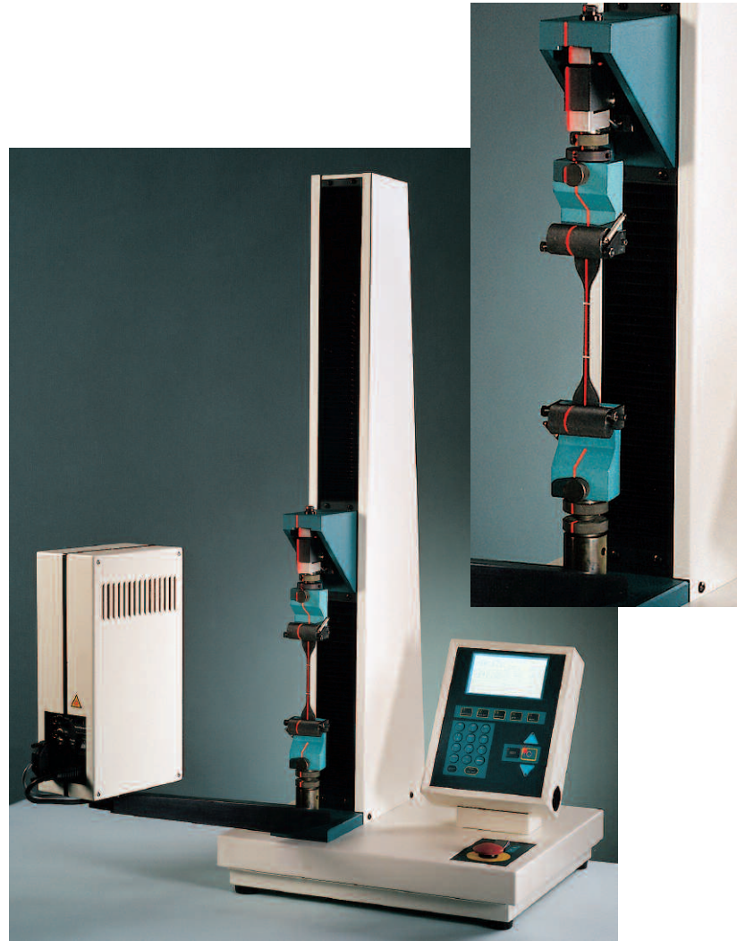
Fig. 3. Model 500LC extensometer mounted on a single column testing machine.
