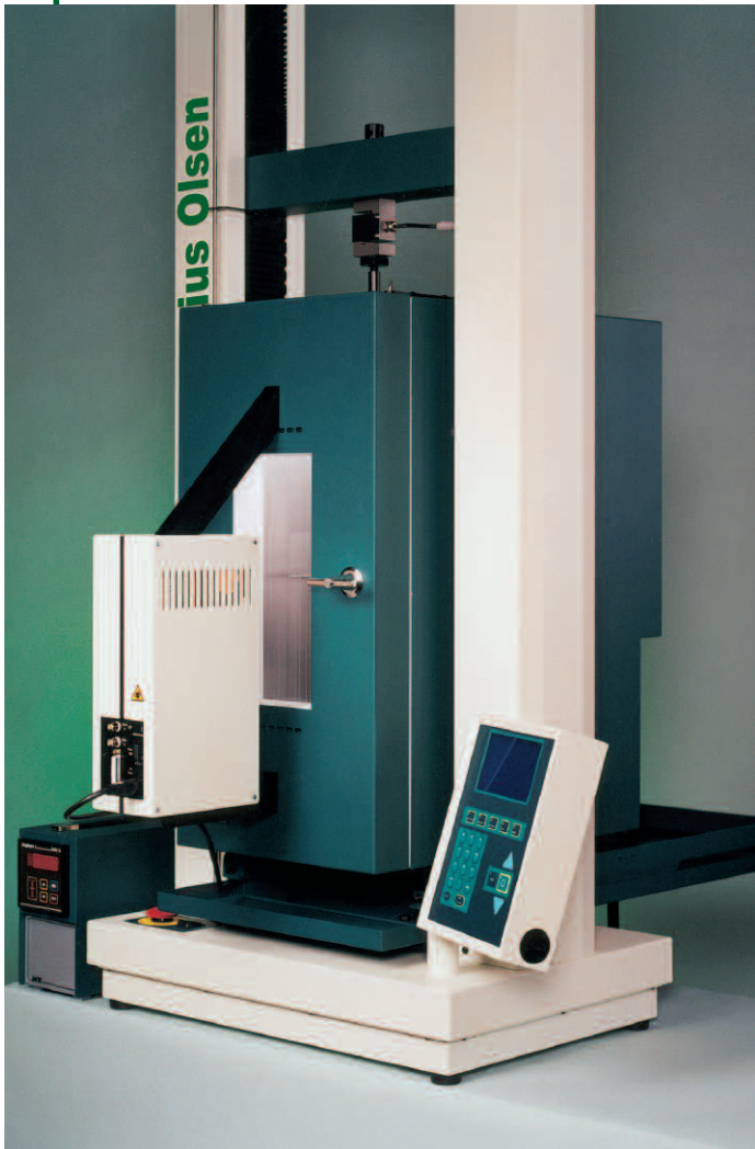
Fig. 2. Model 500LC extensometer mounted on H10kS testing machine with an environmental chamber.
